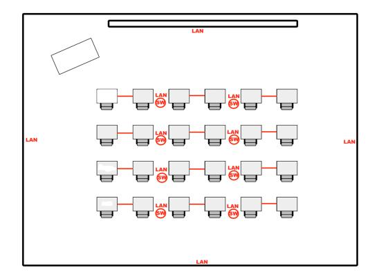
Illustration B: Secondary school layout with eight floor LAN ports connected to multi-port Ethernet switches (SW) mounted under desks. Ethernet cables between desks should be covered with ADA-compliant raceways.
